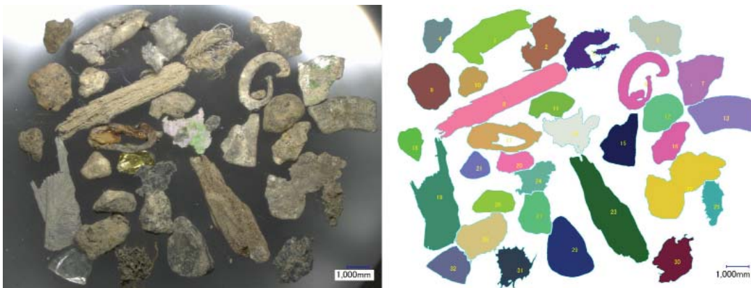
Fig. 2: Example of microscopic images of 1 – 2 mm fraction at 20-fold magnification, front lighting (left) and automated particle segmentation (right).
