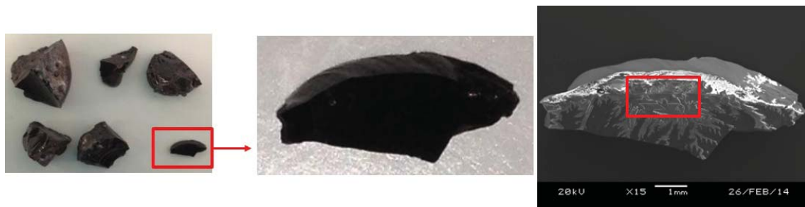
Fig. 4: Slag sample: Fragments (left) und enlargement (middle), Phosphor search Sample, acceleration voltage: 20.0kV, zoom: 10x (right).
