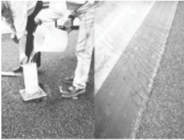
Fig. 8: Testing hydraulic conductivity of steel slag porous asphalt.
