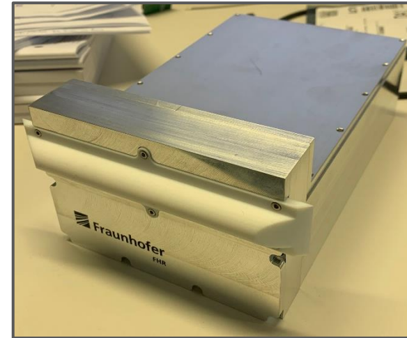
32-channel MIMO Sensor (Antenne designed von IMST GmbH)
